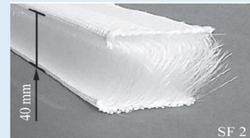
Sample Spacer fabrics used as inserts in the molding tools
